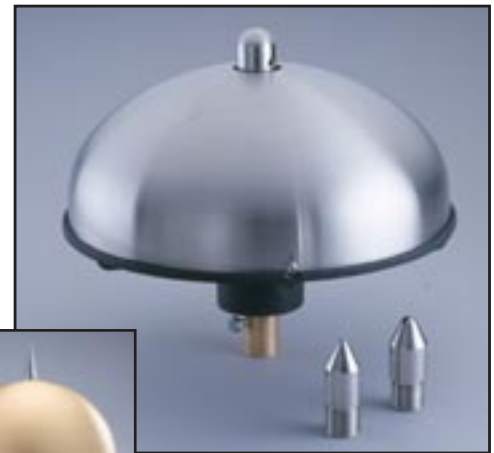
DYNASPHERE Enhanced Air Terminal Capture point of the ERITECH System 3000 initiates an upward leader during thunderstorm conditions to capture lightning discharges over a greater radius than conventional protection.
