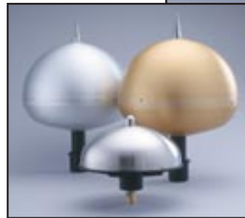
DYNASPHERE Enhanced Air Terminal Capture point of the ERITECH System 3000 initiates an upward leader during thunderstorm conditions to capture lightning discharges over a greater radius than conventional protection.
